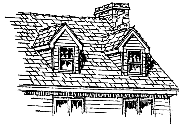
■ Roof lines punctuated by dormers
